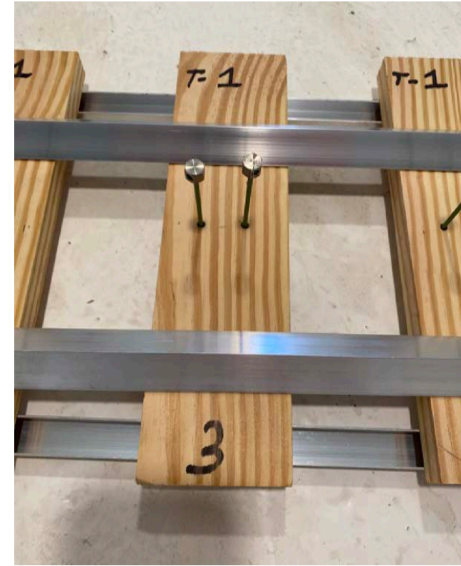
Appendix A4 Figure 5 - Typical probe locations on specimens
