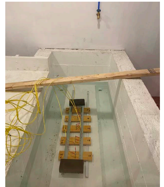
Appendix A4 Figure 8 - Test 1 specimens during flooding
