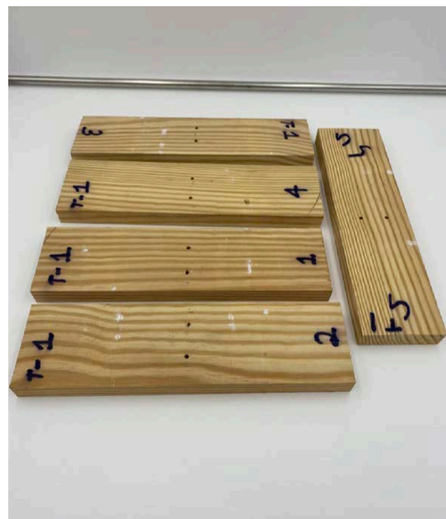
Appendix A4 Figure 11 - Test 1 specimens after drying
