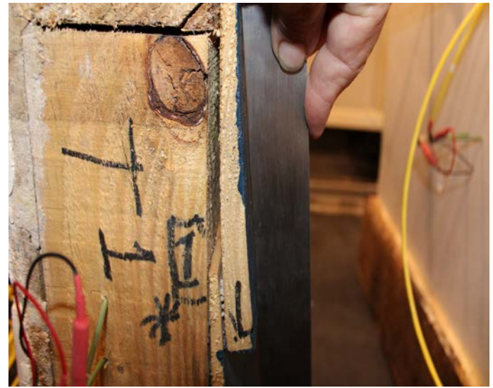
Figures 14 - Sample 1 showing cupped siding against a flat edge.
