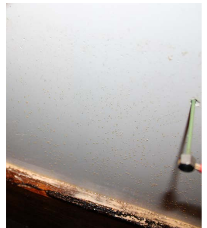
Appendix A3 Figure 16 - Sample 1 crystallized granules on plaster post-draining.
