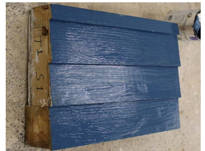
Figure 2 - Sample 1 wall assembly of Plaster on Wood Lath (from top to bottom): "interior" plaster wall, assembly section, "exterior" siding
