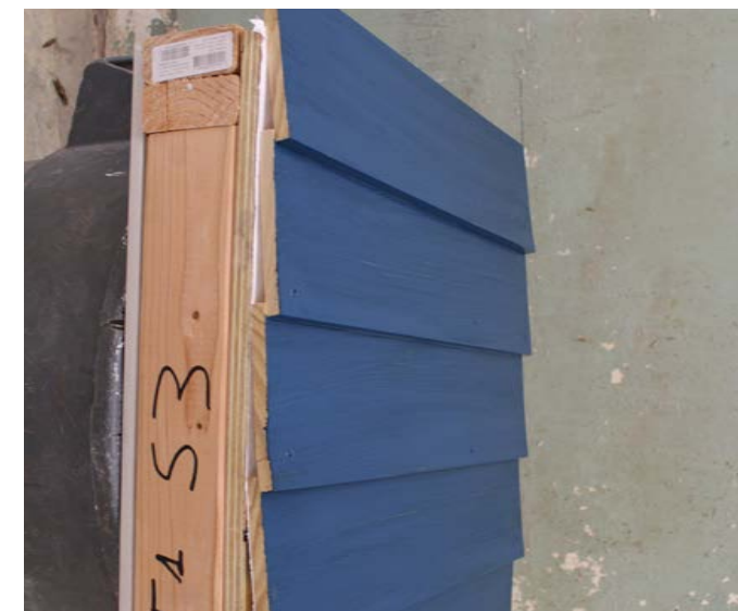
Figure 4 - Sample 3 wall assembly of Modern Drywall (from top to bottom): “interior” drywall, assembly section, “exterior” siding
