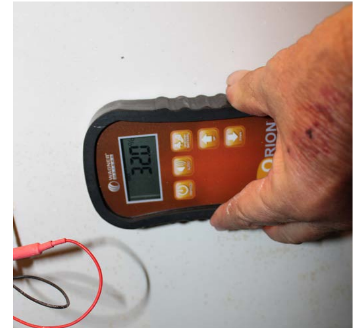
Figure 11 - Measuring moisture content after draining.
