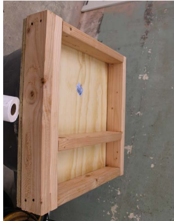
Appendix C3 Figure 2 - Sample 3 construction showing framing.
