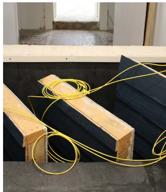
Appendix A3 Figure 11 - Sample 1 (center) in the test chamber with Lignomat probes installed.
