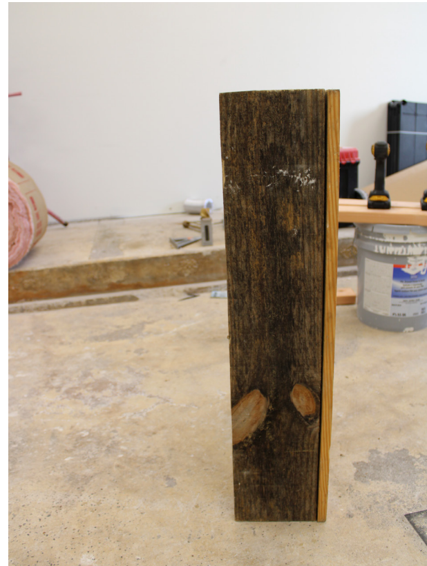
Appendix B3 Figure 2 - Sample 2 construction showing bottom framing.
