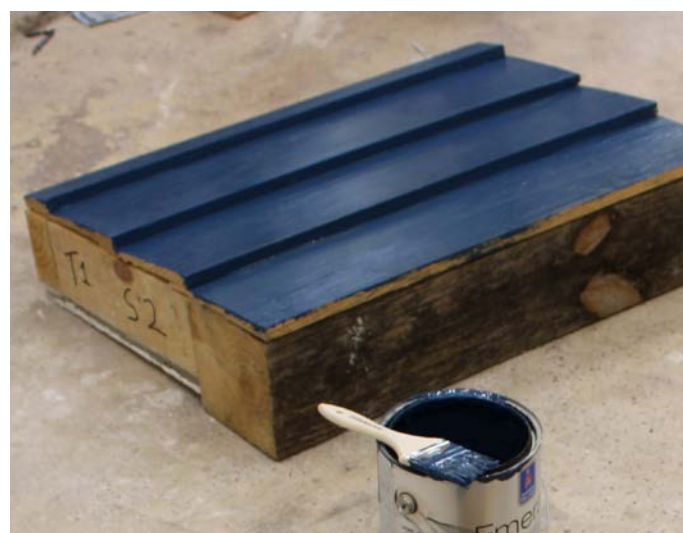
Figure 3 - Sample 2 wall assembly of Plaster on Wire Lath (from top to bottom): “interior” plaster wall, assembly section, “exterior” siding
