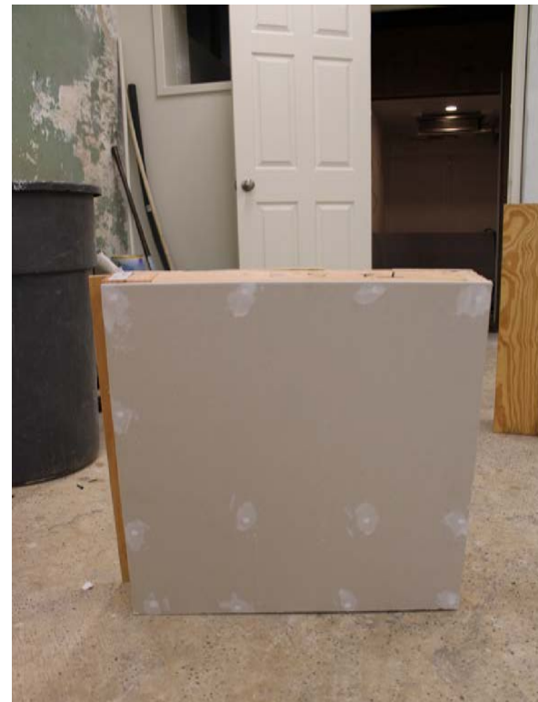
Appendix C3 Figure 7 - Sample 3 construction showing drywall.
