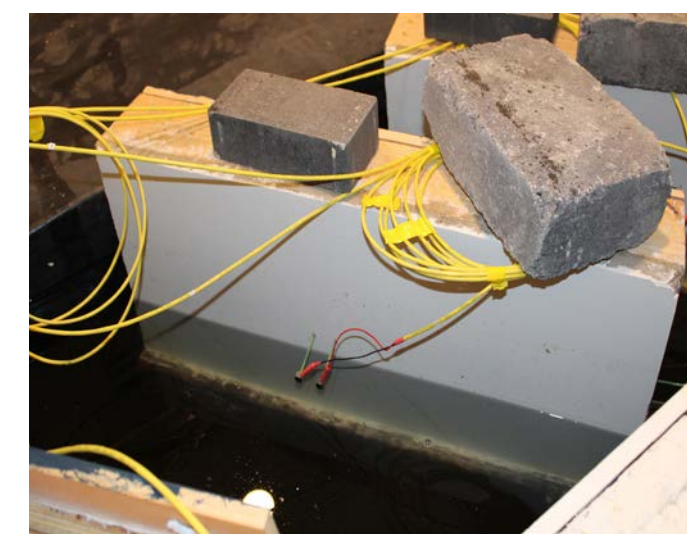
Figure 7 - Test chamber filled with water; flooding assemblies.
