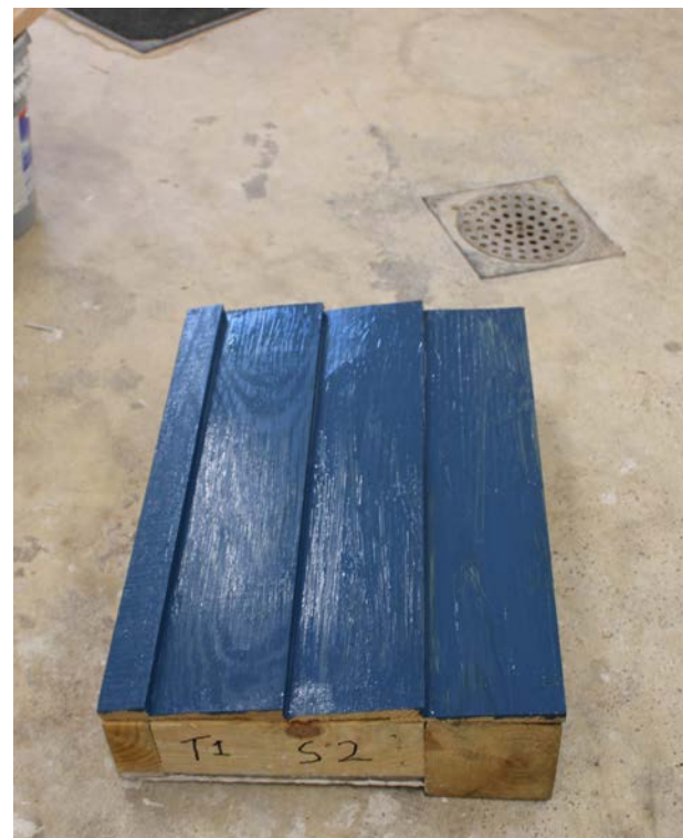
Appendix B4 Figure 4 - Sample 2 construction showing painted taper sawn Southern Yellow Pine siding.
