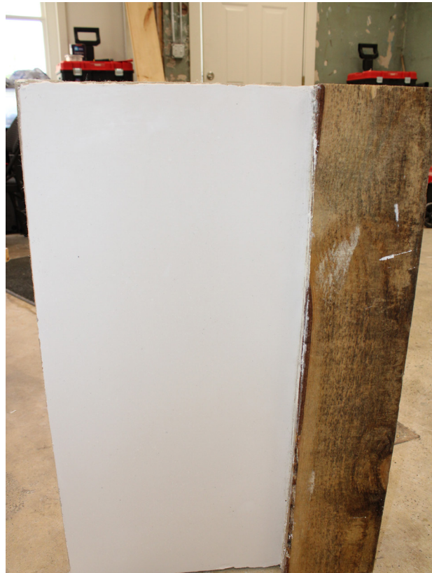
Appendix B3 Figure 1 - Sample 2 construction showing plaster.
