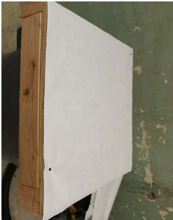
Appendix C3 Figure 3 - Sample 3 construction showing Tyvek wrap.
