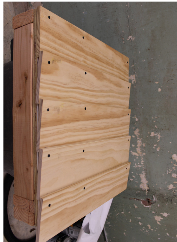
Appendix C3 Figure 3 - Sample 3 construction showing taper sawn Southern Yellow Pine siding.
