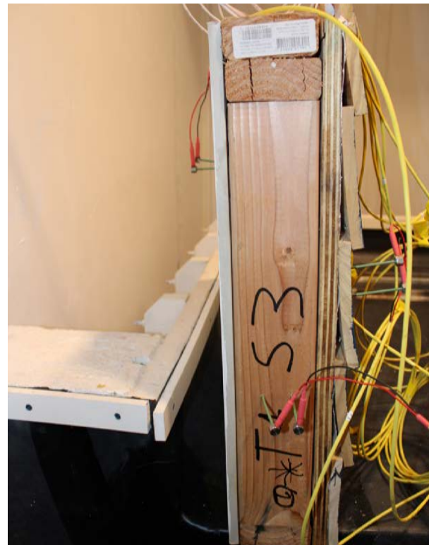
Appendix C3 Figure 12 - Sample 3 during extended drying period with Lignomat probes installed.
