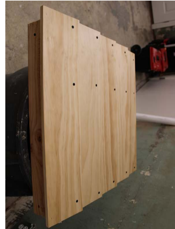
Appendix C3 Figure 5 - Sample 3 construction showing taper sawn Southern Yellow Pine siding.
