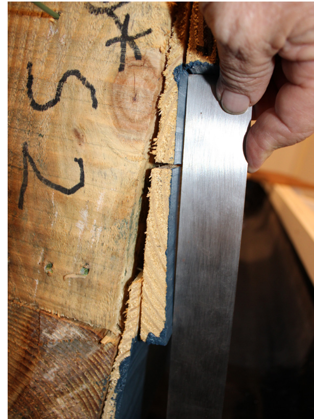
Appendix B3 Figure 13 - Sample 2 showing warping of siding after drying period against a straight edge.
