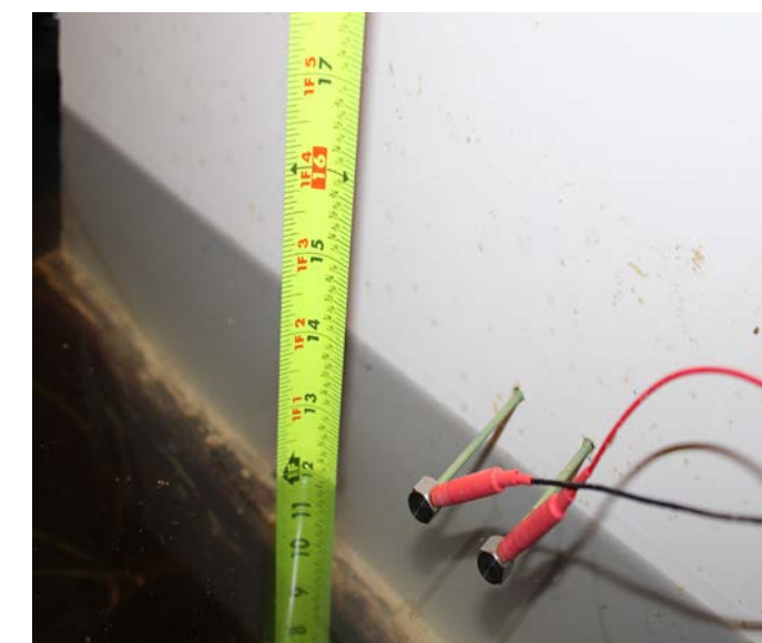
Figure 8 - Detail of measuring water level during flooding.
