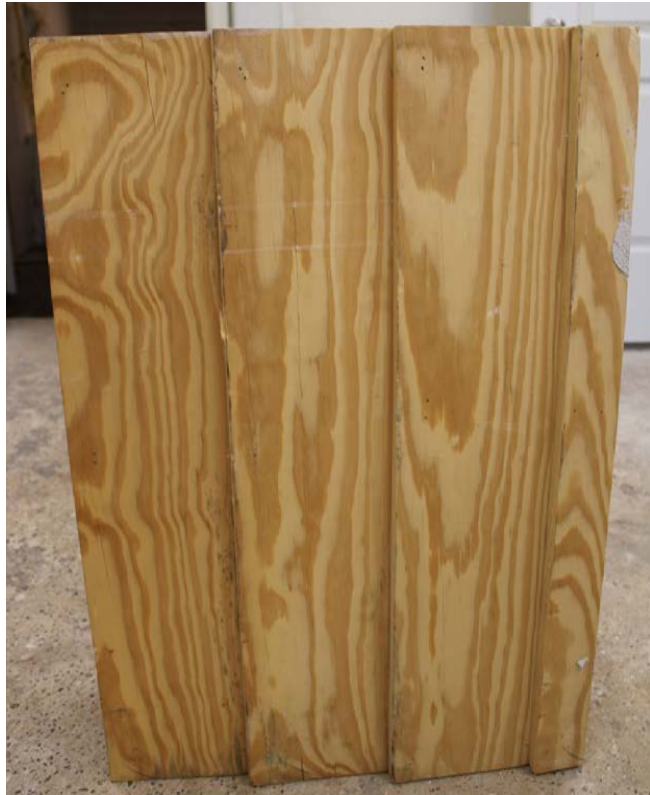
Appendix A3 Figure 1 - Sample 1 construction showing taper sawn Southern Yellow Pine siding.
