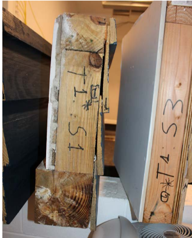
Appendix A3 Figure 17 - Sample 1 during extended drying period.
