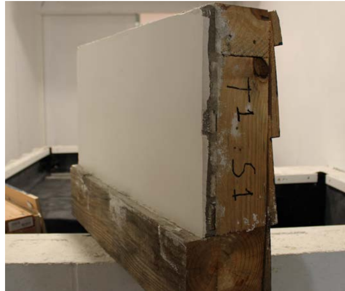
Figure 12 - Sample 1 assembly prior to flooding.
