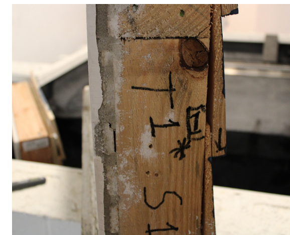
Detail of wood lath and plaster wall assembly
